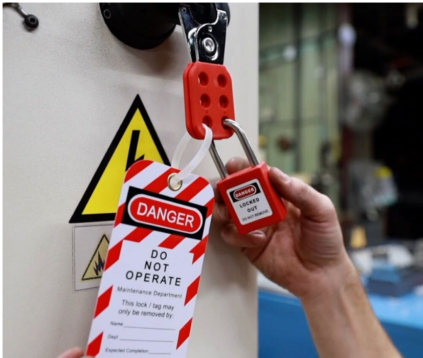
Figure 6-9: Logout – tagout system in place 38
