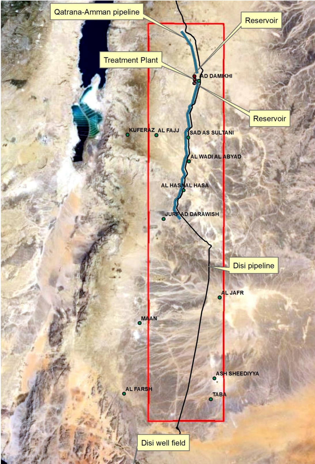
Figure 1: Proposed water supply infrastructures
