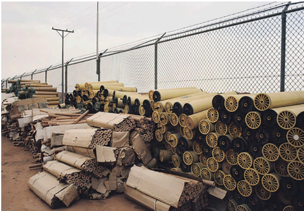
Figure 1-24: Used reverse osmosis spiral wound modules and cartridge filters pile up outside a RO plant
